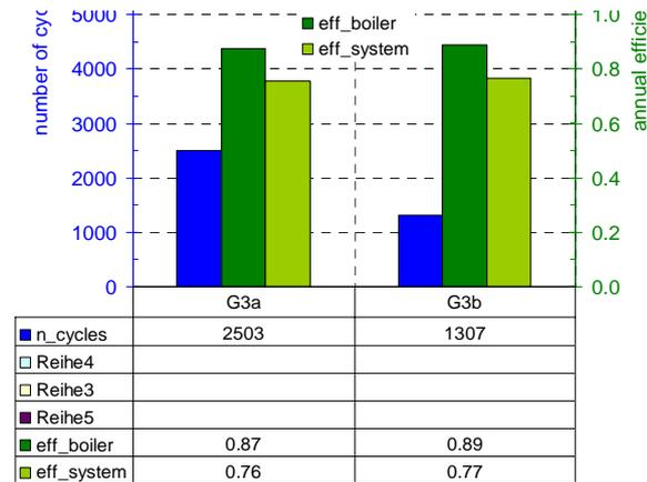
Figure 4: Annual number of start-stop cycles and annual efficiency for the systems G3a (water storage) and G3b (bulk PCM storage)
