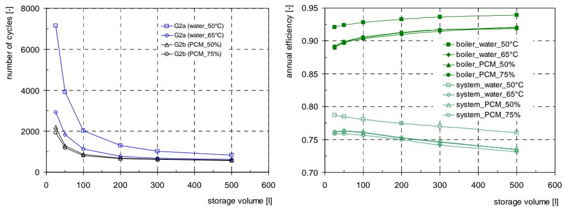
Figure 3: Gas boiler: annual number of start-stop cycles (left) and annual efficiencies (right) for different storage volumes for systems with water storage (G2a) and for systems with water storage with integrated PCM modules (G2b)
