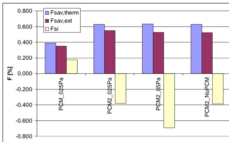
Figure 6: Difference of heat storage with makroencapsulated PCM with various sensor and in/outlet positions and a sole water store.
