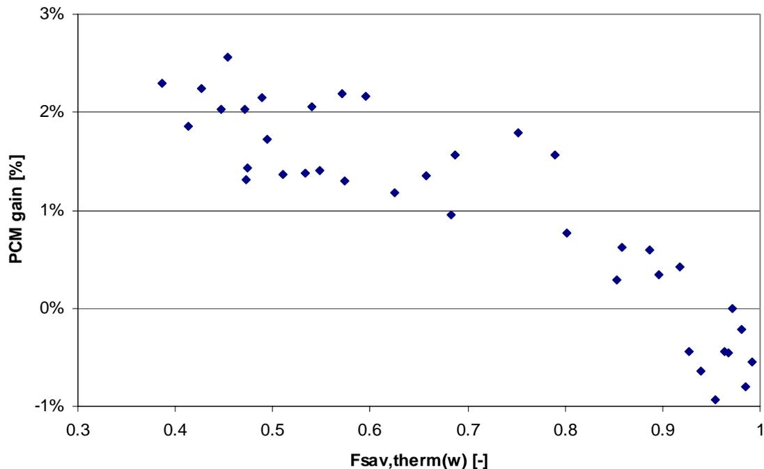
Figure 1: Difference between sole water and water + PCM system. The PCM gain =  $F_{sav,therm(W+PCM)}/F_{sav,therm(W)} - 1$
