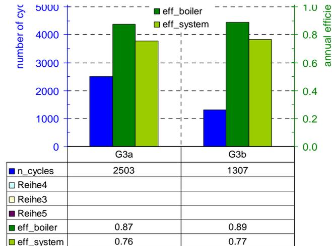
Figure 5: Annual number of start-stop cycles and annual efficiency for the systems G3a (water storage) and G3b (bulk PCM storage)
