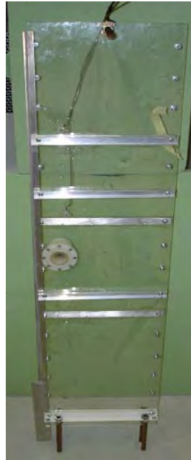
Figure 3.2. Modified design. On one side the gap is closed, the inlet is positioned near the closed side but vertically centred. Traverses assure flatness of the plastic material.
