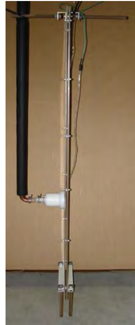
Figure 3.3. The modified design viewed from the side. The supply pipe is made of copper, with an outer diameter of 12 mm, insulated with EPDM foam.
